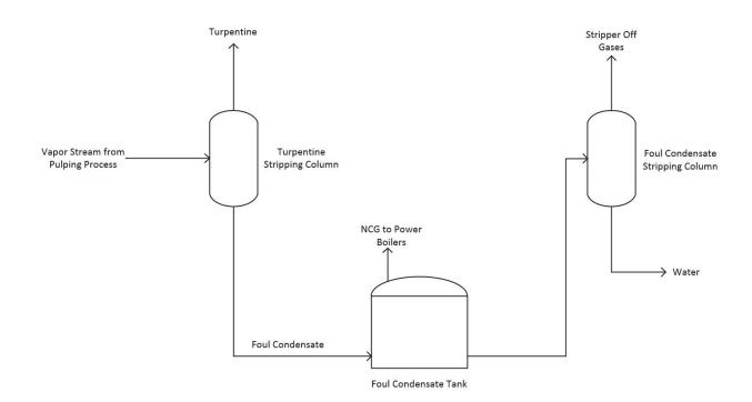
**Figure 3.** Simplified Flow Diagram of the Foul Condensate Tank. The foul condensate tank is fed by the turpentine-stripping column and then sends foul condensate to the foul condensate-stripping column.
