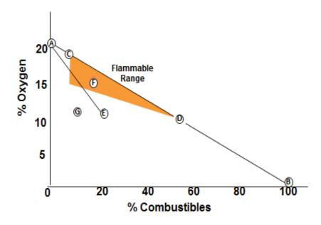
**Figure 6.** Typical Flammable Range of NCG. The highlighted area between points C and D represents mixtures of NCG and oxygen that are flammable [5, pp. 4-5], [6]. The flammable range can change substantially with the addition of turpentine.
