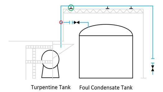
**Figure 13.** Simplified Drawing of the Scope of Work Conducted on the Water Piping. The scope of work on the water piping required three tasks: (1) disconnect and move water piping back onto its piping rack, (2) fix a crack in the water piping at the intersection of the three-inch line that connected to the foul condensate tank (smaller red circle), and (3) weld a guide onto the piping rack to prevent the water piping from slipping off of the pipe rack in the future (larger green circle).
