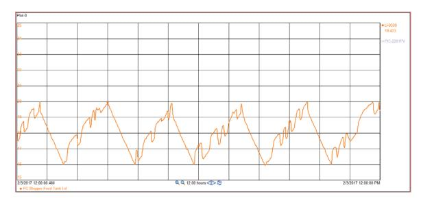
**Figure 20.** Plot of the Foul Condensate Tank Level Showing the Typical Cycle to Skim Turpentine by Using the Tank's Internal Weir. The tank level has a range of 15 to 25 feet of liquid. Automatic controls were installed to cycle the tank level from 16 to 20 feet to skim turpentine into the tank weir system.
