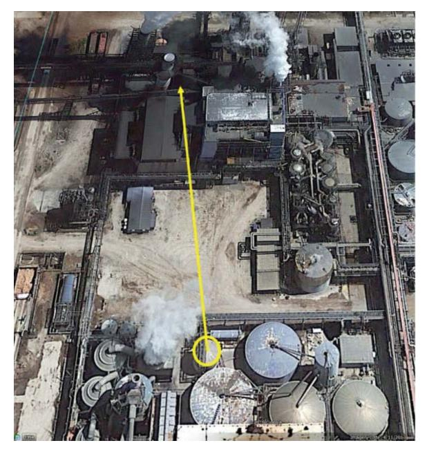
**Figure 8.** Overhead Photograph of the PCA DeRidder Mill. The yellow circle shows the preincident location of the foul condensate tank and the yellow line indicates the path traveled by the tank following the explosion. The tank landed at the base of a powerhouse stack, as indicated by the arrow. Photograph: Google Earth.
