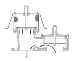
**Figure 25.** Relief/Protection Functions of the Pressure Vacuum Breaker. The image at the left shows that as pressure in the vessel increases, a pressure pallet lifts and relieves tank pressure to the atmosphere. The image at the right shows that as a vacuum is drawn into the vessel, the vacuum pallet lifts and air is drawn into the vessel from the atmosphere. Image: Groth Corporation [13].
