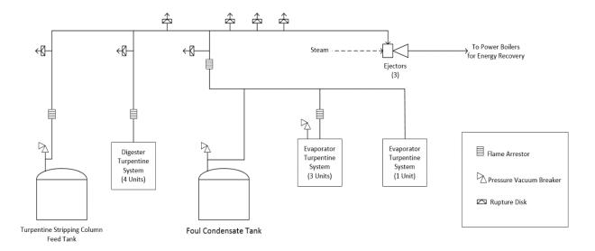
**Figure 43.** Simplified Flow Diagram of the CNCG System Showing the Interconnection Between the Foul Condensate Tank and the Turpentine System. The turpentine system is composed of the evaporator turpentine system, and the digester turpentine system.
