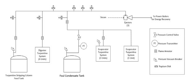
**Figure 4.** Simplified Flow Diagram of the CNCG System. The CNCG system collects NCG from various units at the mill, including the foul condensate tank, and sends them to the power boilers for energy recovery.
