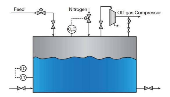
**Figure 37.** ARCO Chemical Wastewater Tank. "The 900,000-gallon wastewater tank had a nitrogen purge to keep the vapor space inert and an off-gas compressor to draw off hydrocarbon vapors before waste disposal." Credit: [42].
