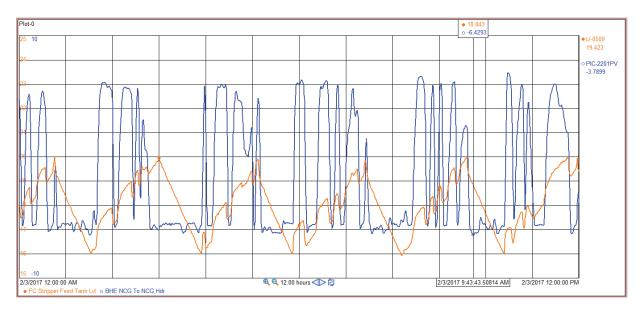
**Figure 26.** Process Data Trend Showing Typical Pressure and Level of the Foul Condensate Tank During Operation. The tank level is shown by the orange trend line with a range of 15 to 25 feet of liquid. The tank pressure is represented by the blue trend line and ranges from approximately - six to + six inches of water, which are the set pressures of the pressure vacuum breaker (the limits of the graph are 10 inches of water vacuum to 10 inches of water pressure).<sup>b</sup>
