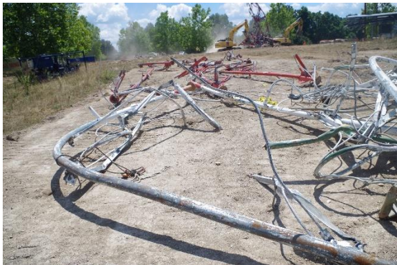
Figure 8. Bent Tower Leg from the Recovered Section
