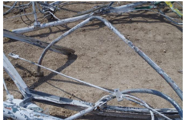
Figure 9. Bent Redundant Member at 105' Tower Elevation
