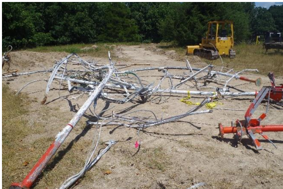
Figure 7. Recovered Section of the Tower 90'-120'
