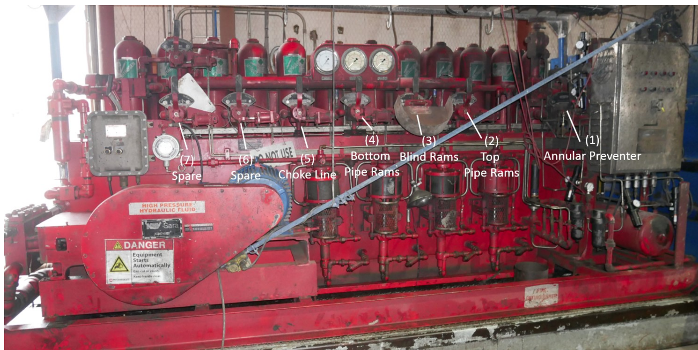
Figure 31. Photo of the BOP accumulator, which is used to function the BOP rams. The rig manager closed the BOP control handles in the following order: (1) annular preventer, (2) top pipe rams, (3) blind rams, and (4) bottom pipe rams. The blowout preventer did not seal the well to stop the blowout when the rig manager functioned the control handles.
