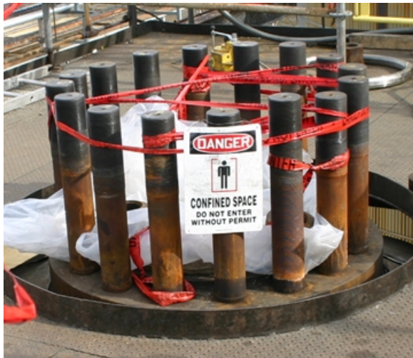
Figure 11. Confined space warning sign on the unsecured reactor manway after the incident.
