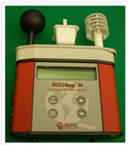
Figure 2. Quest WBGT meter with natural wet-bulb sensor
