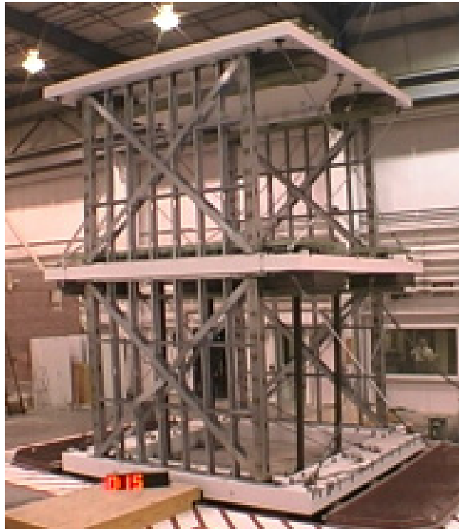
Figure 8-53. Overall view at largest positive cycle, 100% SE32 test near 15.7 sec.
