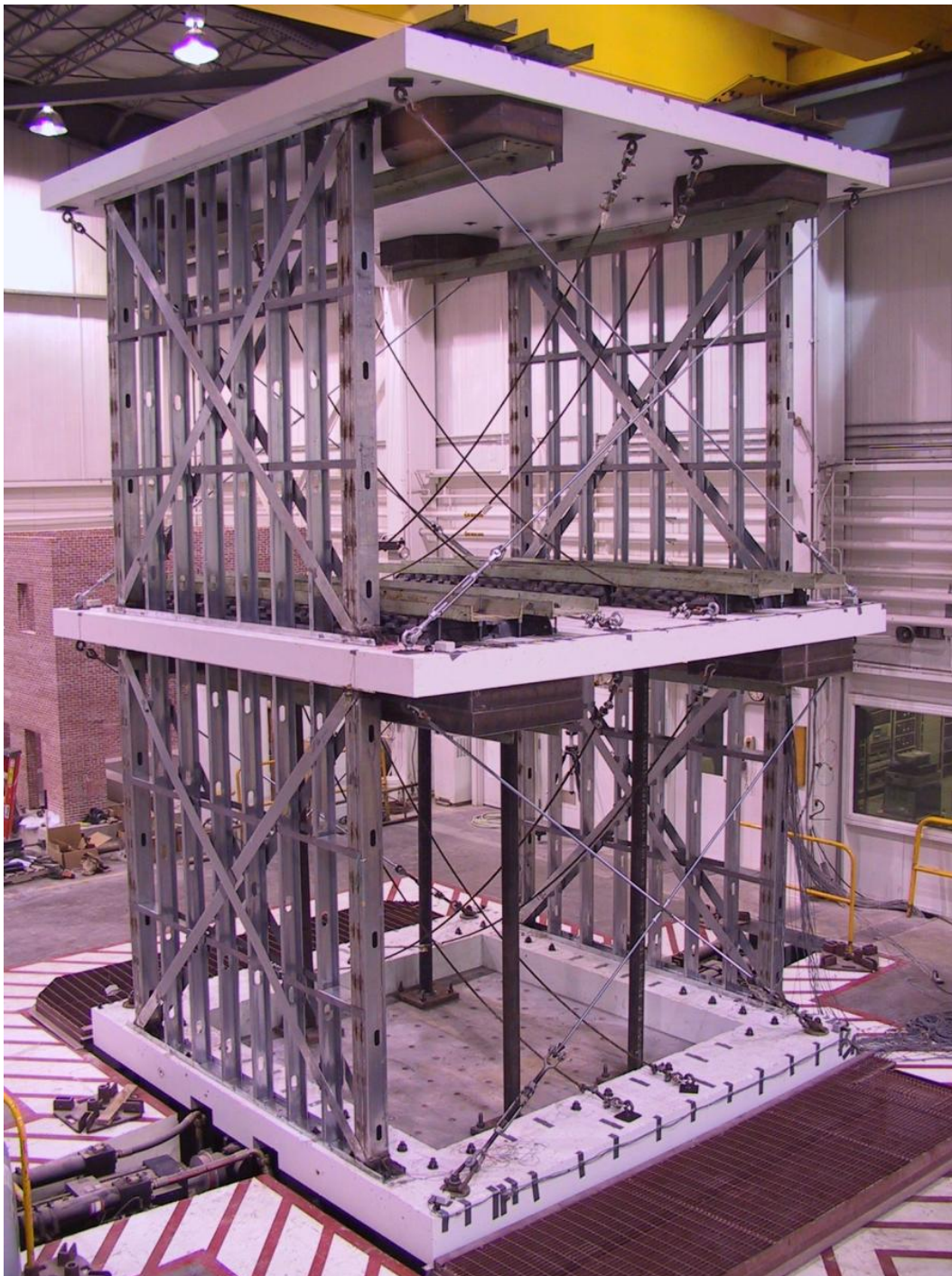
Figure 8-1. Photograph of the cold-formed steel verification model mounted on the ERDC-CERL TESS (viewed from northeast corner).
