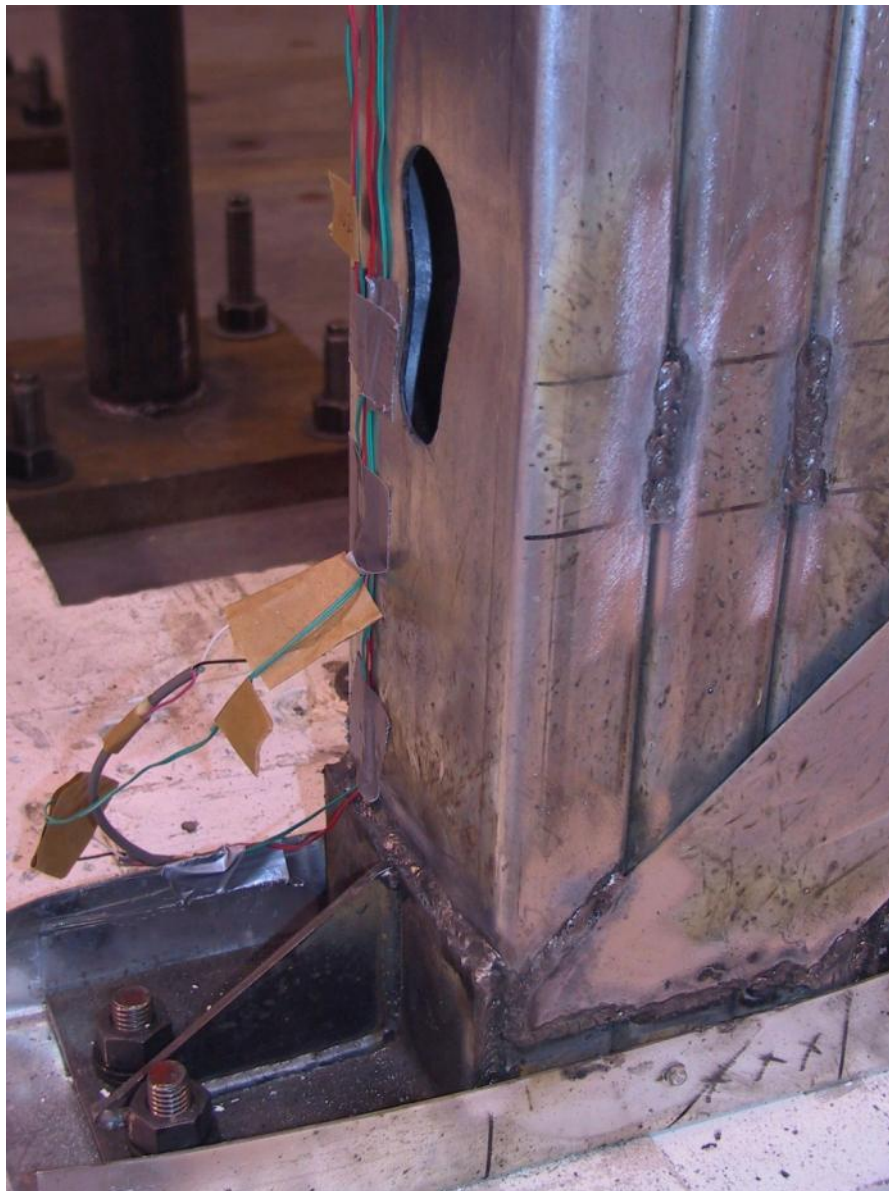
Figure 8-67. Bottom of southeast column facing west, showing local column buckling and anchor and column bending at top of the anchor.
