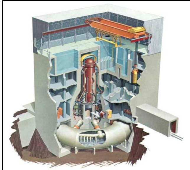
Figure 3. GE BWR / Mark I Containment Structure (Showing Torus Suppression Pool)
