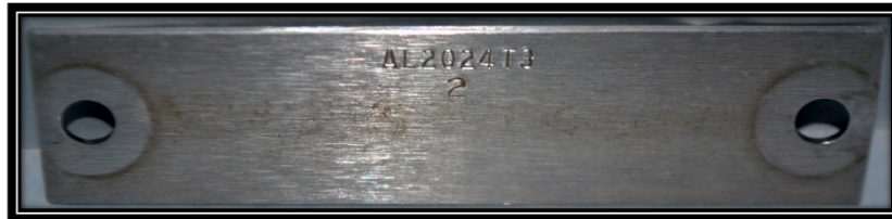
Figure 3: AL2024 T3 Sample prior to Corrosion Removal
