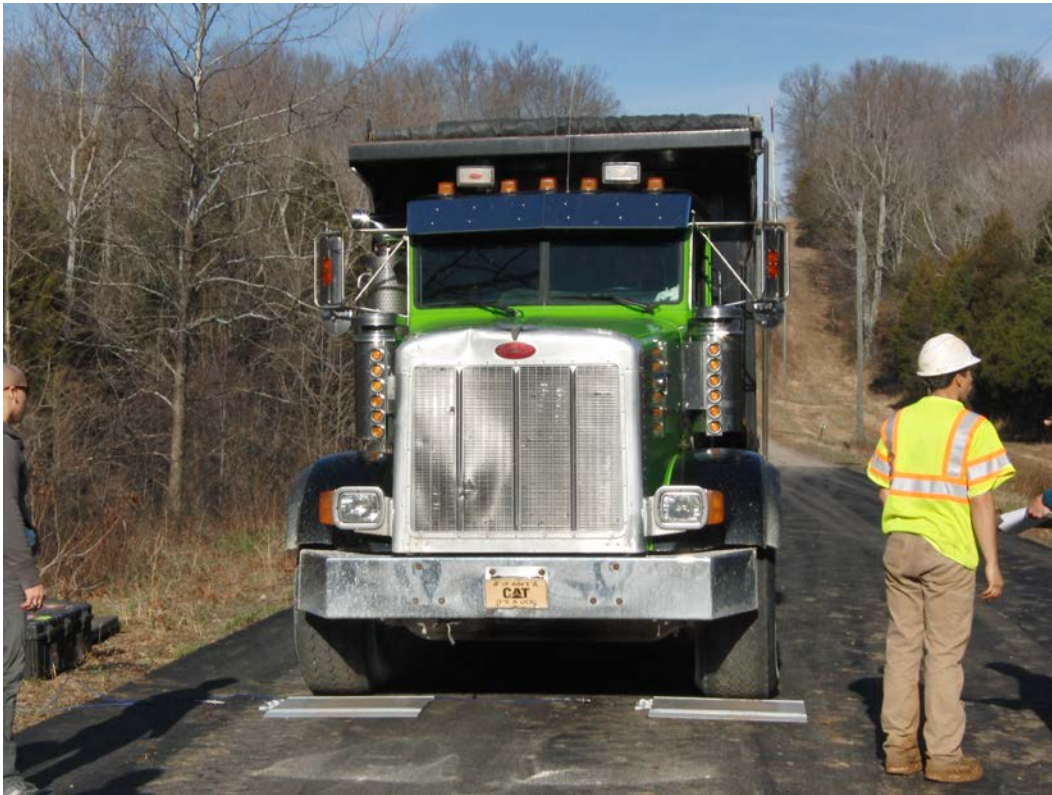
Figure 17. Weighing a truck to be used for load testing.
