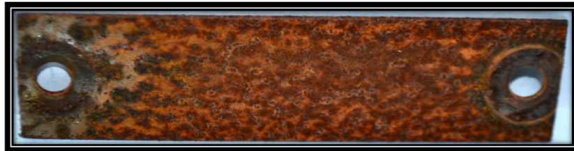
Figure 7: C1010 Sample prior to Corrosion Removal
