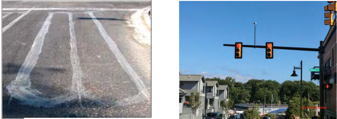
Exhibit 1-2. Vehicle detection by inductive loop (left) and video (right) (Source: Left: South Carolina DOT / Right: Jeff Shaw, FHWA)
