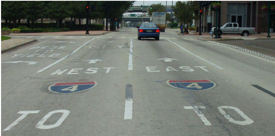
Exhibit 5-23. Example of pavement legends indicating destination route numbers (“horizontal signing”).
