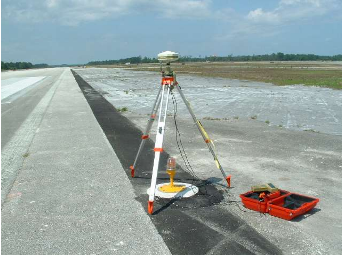
Figure 2-3. Airfield NAVAID positioning using Fast-Static GPS methods
