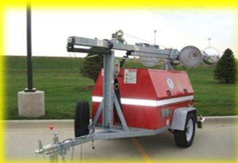
Recently, an agency received a safety notice from the Department of Labor concerning fraying on a cable on the generator light tower. The cable is part of the light standard raising/lowering mechanism. Please take a moment to visually inspect this cable. Divisions should contact their Branch Chief with any questions regarding MABAS assigned resources.
