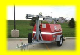
Recently, an agency received a safety notice from the Department of Labor concerning fraying on a cable on the generator light tower. The cable is part of the light standard raising/lowering mechanism. Please take a moment to visually inspect this cable. Divisions should contact their Branch Chief with any questions regarding MABAS assigned resources.
