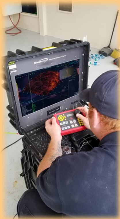
ROV Technician "flying" the unit using the sonar display
