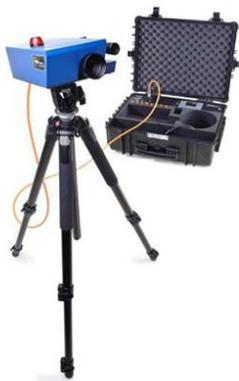
Lazer operated safety device that monitors building movement during Technical Rescue / Structural Collapse Operations.
