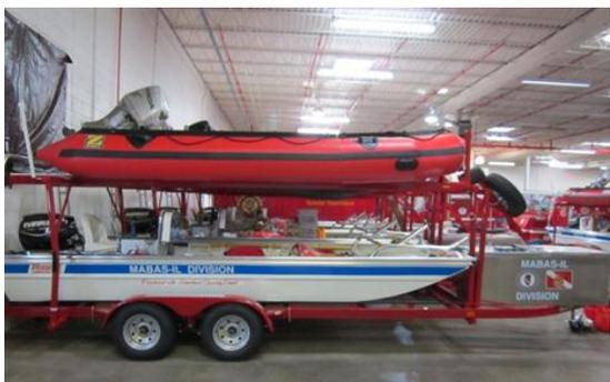
One inflatable and one rigid hull boat with 40 hp motors and safety/rescue equipment
