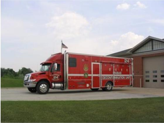
**Capabilities:** Mass decontamination – up to 200 people with supplies on board. Shower and hygiene facilities. Exterior, under-awning, misting nozzles for cooling.
