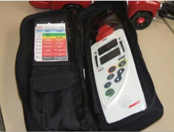
Portable, battery operated carbon monoxide meter. Analyzes the percentage of oxygen and CO levels in the blood.
