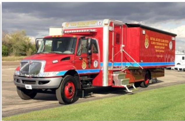
Mobile office space for Incident Command function, credentialing, etc. On board generator, heat, A/C, etc. 4 Units Statewide.
