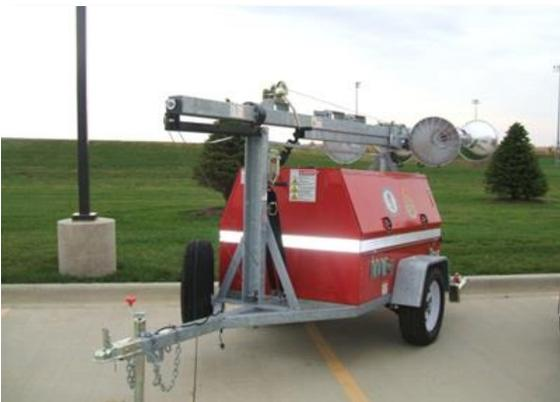
20 Kw diesel-powered with 4 – 1000 w floodlights.
