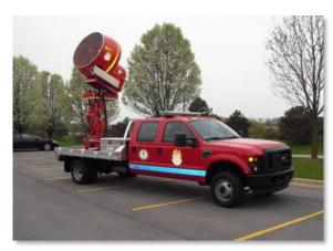
100 hp fan motor on elevating, rotating, and tilting stalk. Used for hi-rise ventilation, confined space ventilation, mass decontamination/cooling (with attachment for hose), toxic gas dissolution, etc.
