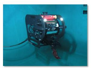
Remotely operated underwater high-resolution imaging device, sonar helps locate and navigate to victims even in zero visibility; allows operator to manipulate interlocking saw to retrieve victims or evidence.
