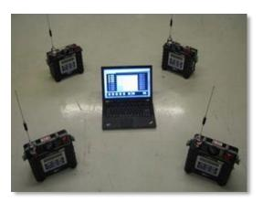
Monitors/analyze air quality and travel distance of unknown "plume" of a hazardous material in and around an incident.
