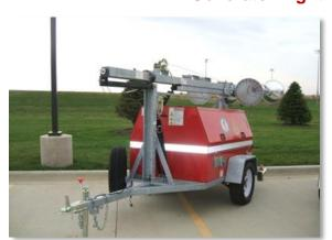
20 Kw diesel-powered with 4 - 1000 w floodlights.
