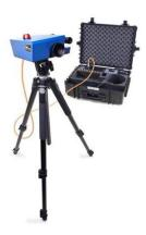
Lazer operated safety device that monitors building movement during Technical Rescue / Structural Collapse Operations.
