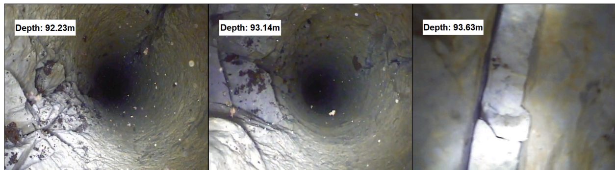
Fig. 8. Borehole S3-Pa as captured by down-hole camera footage: Images showing a geological structure at varying depths.
