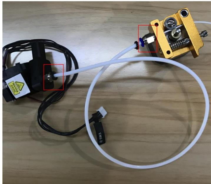
Figure 5.121 Connect extruder and hot end
