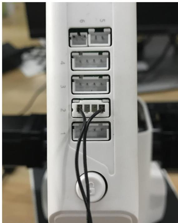
Figure 5.171 Insert the cable of the auto-levelling
