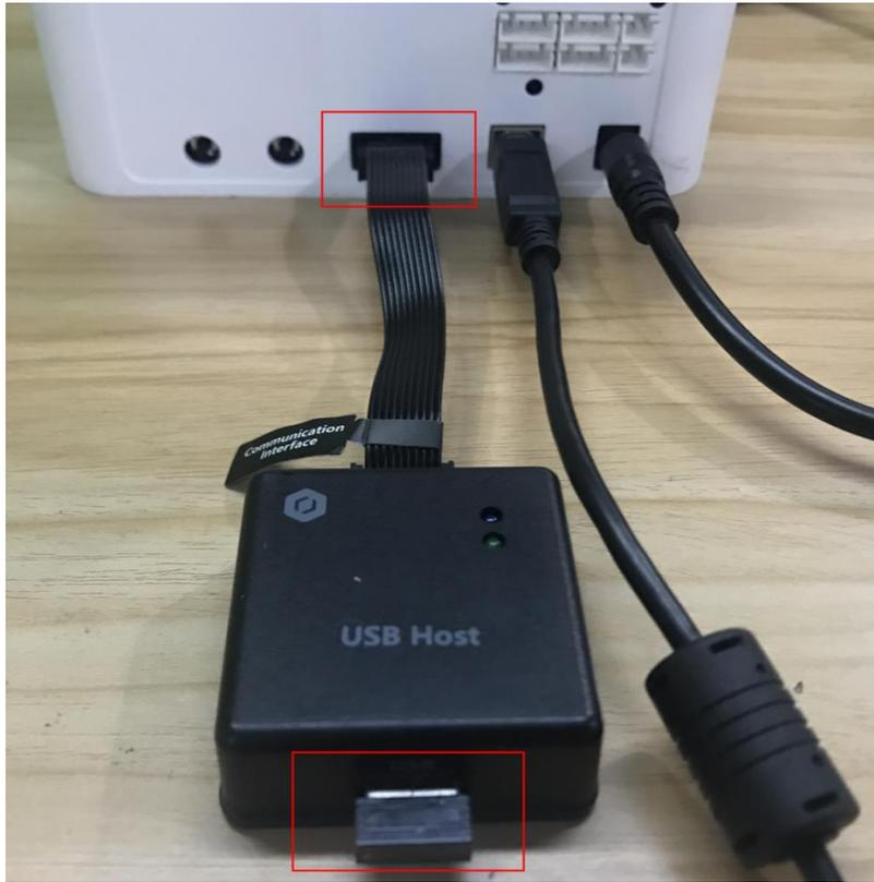
Figure 5.186 Connect with USB Host module
