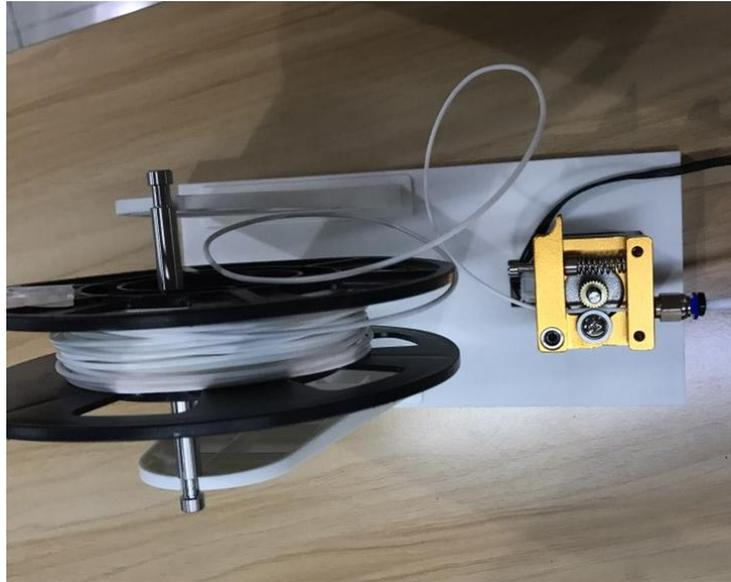
Figure 5.125 Place filament and extruder to the Filament holder
