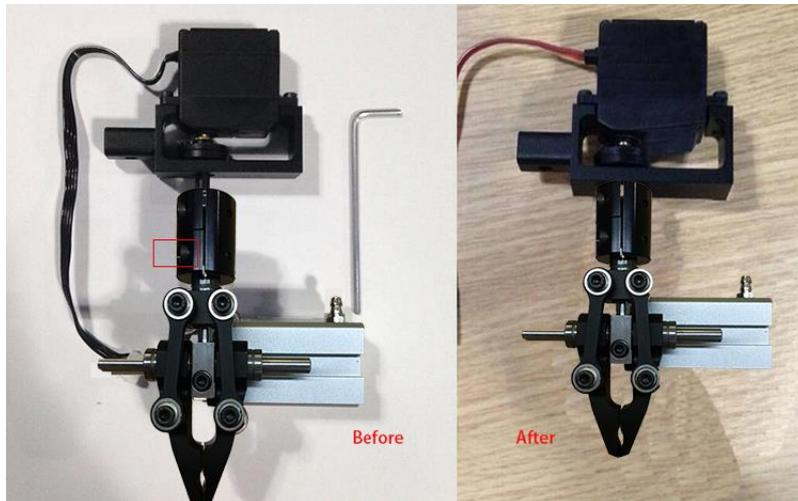
Figure 5.13 Install a gripper kit
