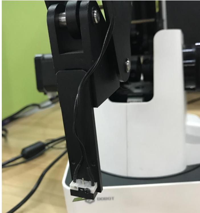
Figure 5.170 Fix auto-levelling tool
