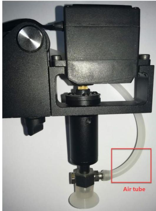
Figure 5.9 Install an air tube
