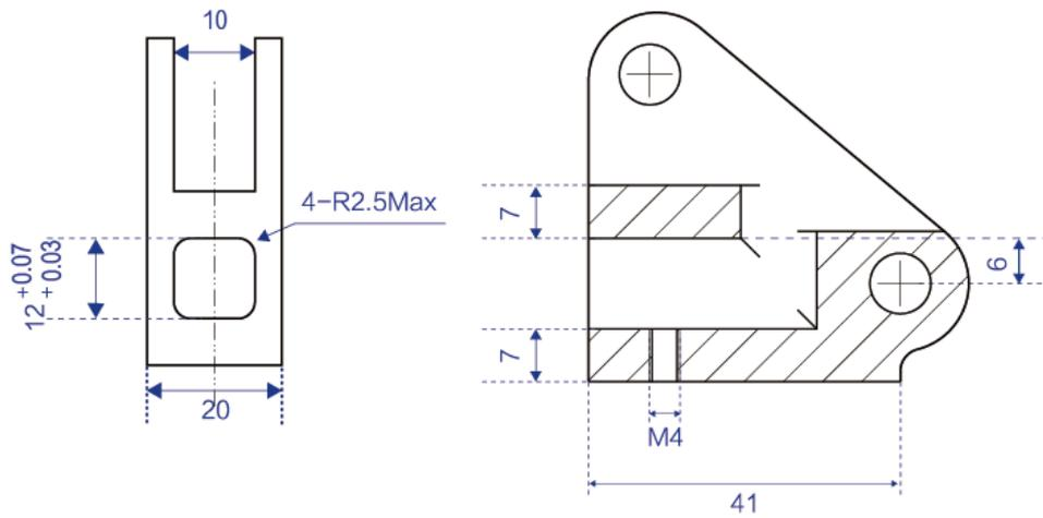
Figure 3.10 Size of end mounting hole
