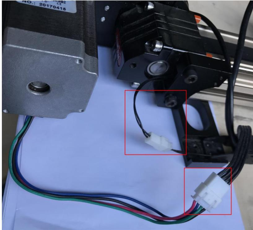
Figure 5.196 Connect sliding rail and wire set
