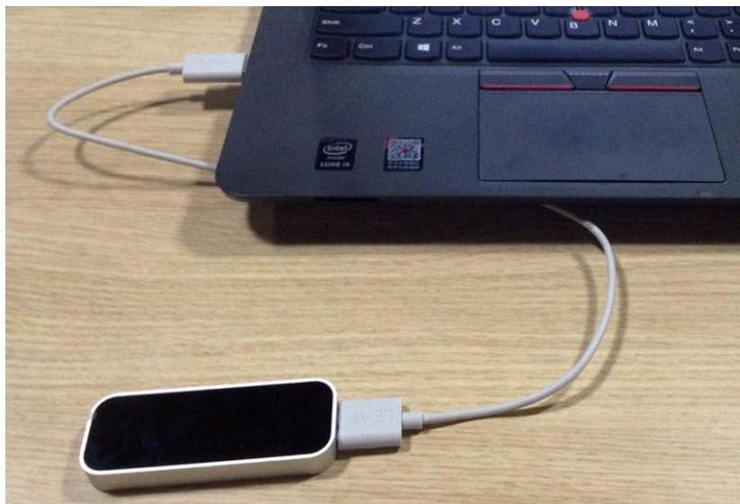
Figure 5.107 Connect the Leap Motion controller to your computer
