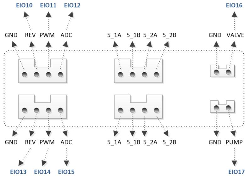
Figure 4.4 Peripheral Interface
