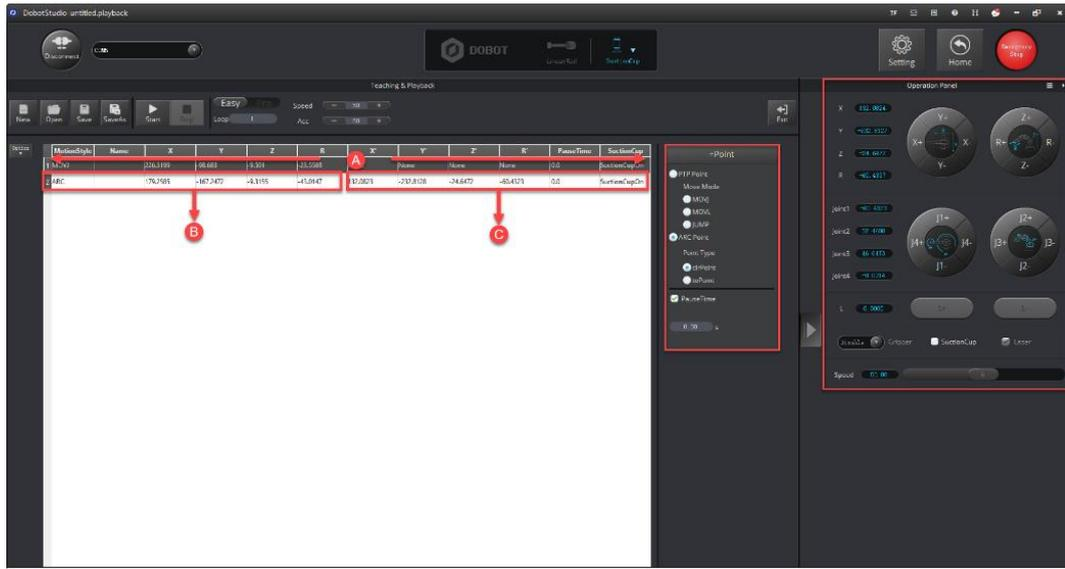
Figure 5.23 Save the second position B and the end position C
