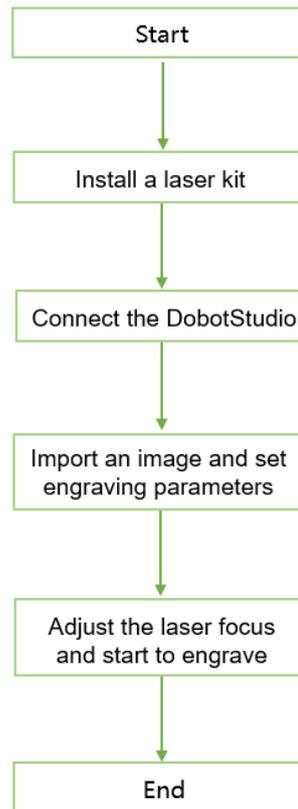
Figure 5.86 The process of engraving a grayscale image
