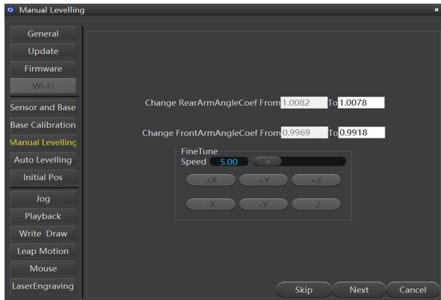
Figure 5.161 Get the angle sensor coefficients
