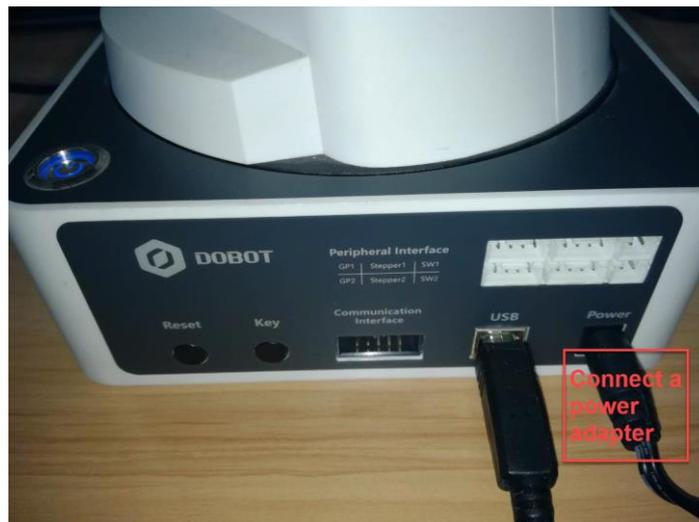
Figure 2.3 Connect the Dobot Magician to the electrical outlet
