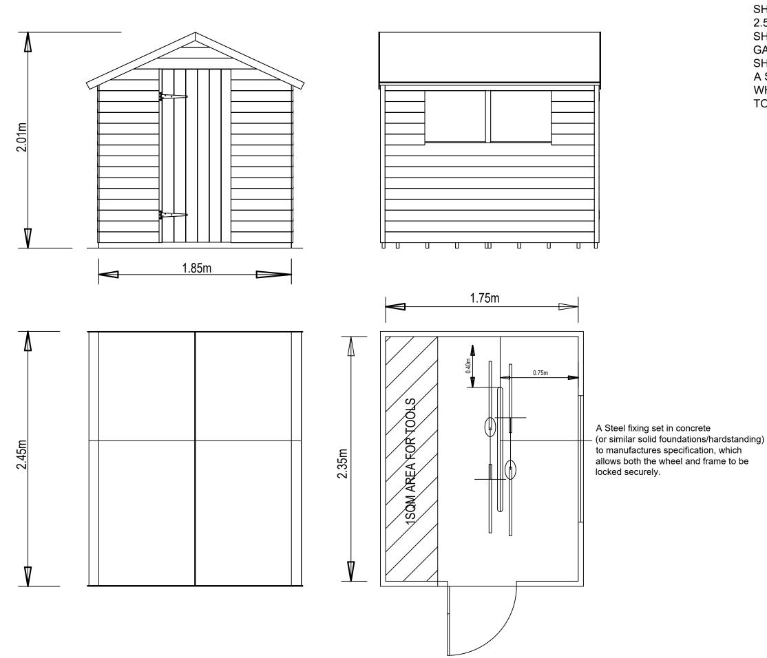
7FT X 5FT TONGUE AND GROOVE TIMBER SHED. DIP TREATED SOFTWOOD. STERLING BOARD ROOF AND FLOOR. 2 PERPEX WINDOWS. SHED TO HAVE A MINIMUM INTERNAL AREA OF 2.5M2. WHEN PROVIDING CYCLE STORAGE IN A SHED A MINIMUM OF 1SQM IS REQUIRED FOR GARDEN TOOLS.
