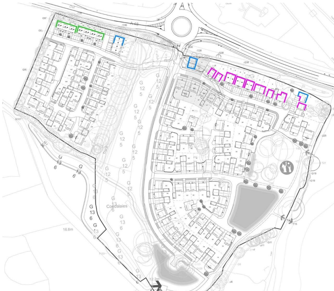
Figure 5.1 – Façades Requiring Additional Sound Insulation Measures
