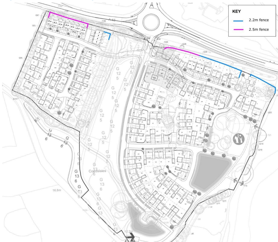
Figure 6.1 – Increased Height Closed Board Fences
