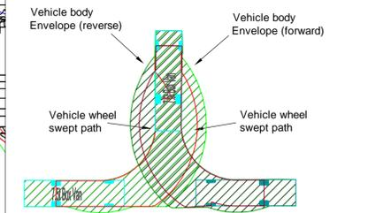
Vehicle Chassis, shown at start & end of path and change of direction(forward).
