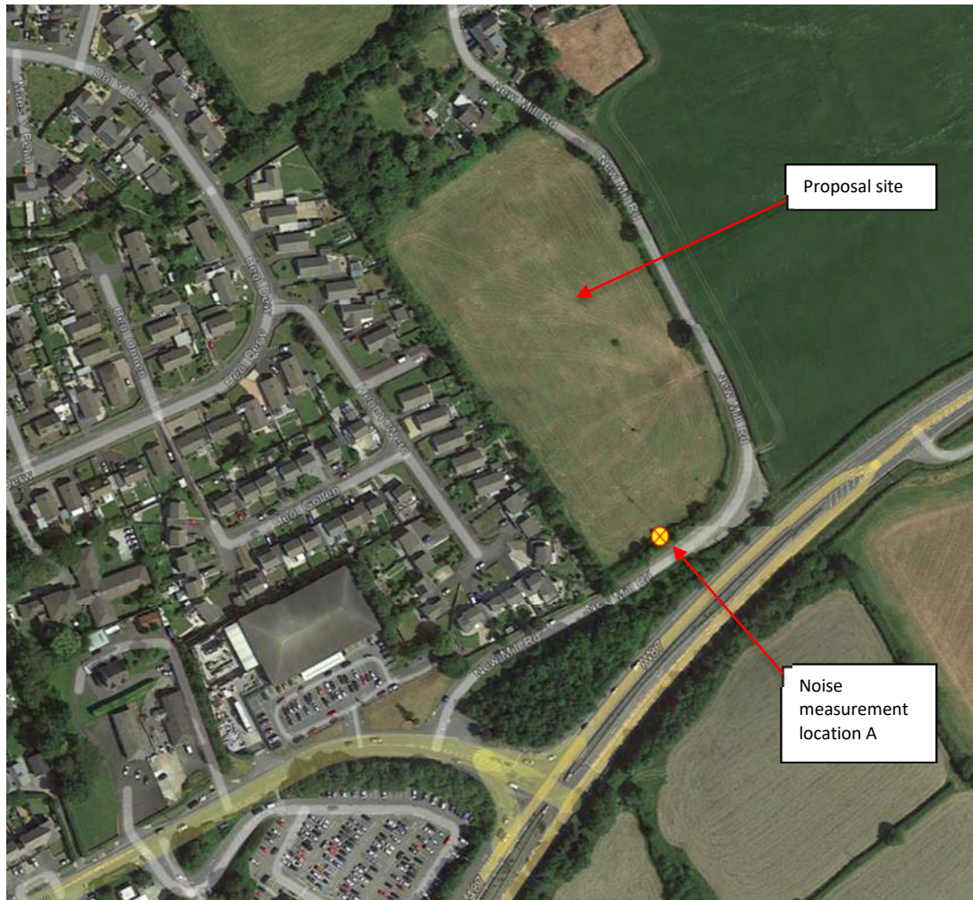
FIGURE 3: Noise measurement location
