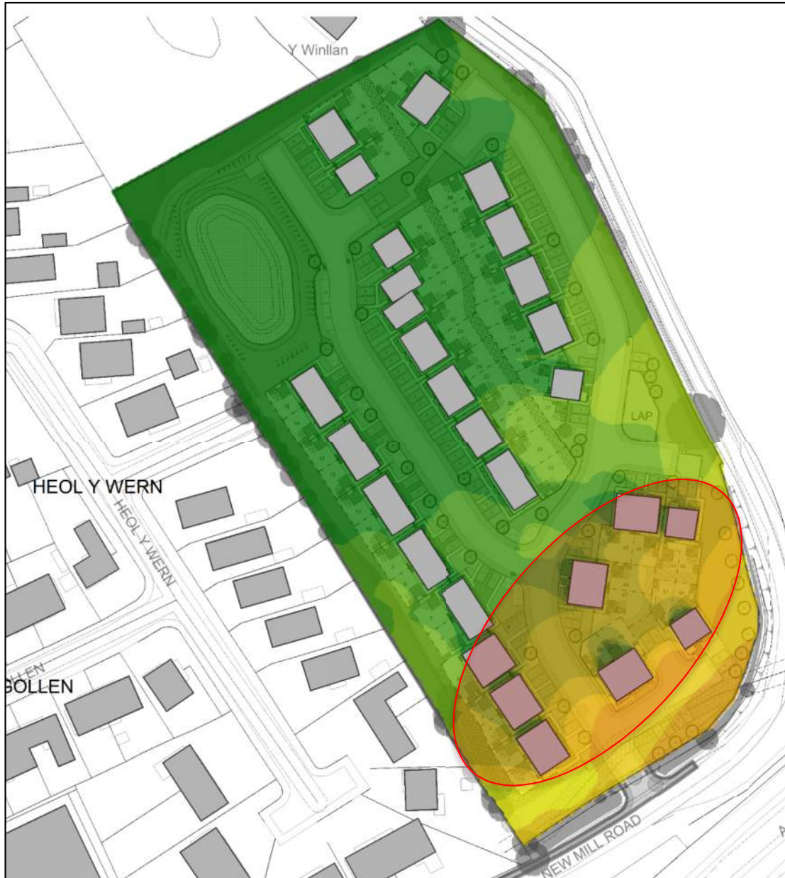
FIGURE 6: Extent of plots requiring closed windows to meet BS 8233 internal noise levels
