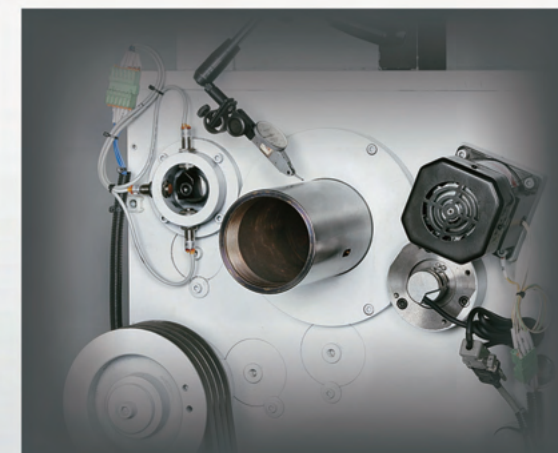
Spindle run-out inspection at the rear end
