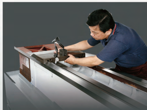
Straightness inspection on bed slideways
