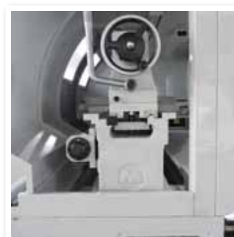
Meehanite Licensed Casting Bed
