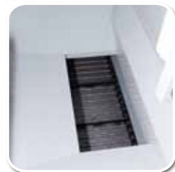
Drainage outlet & Chip conveyor
