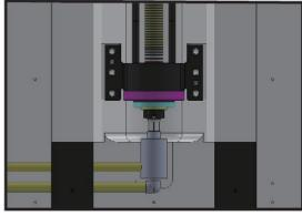
Z axis precision ballscrew with coolant through design to reduce thermal expansion error
