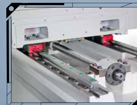
Linear Guideways suitable for fast cutting to ensure the fine cutting surface and quality for high precision requirement.
