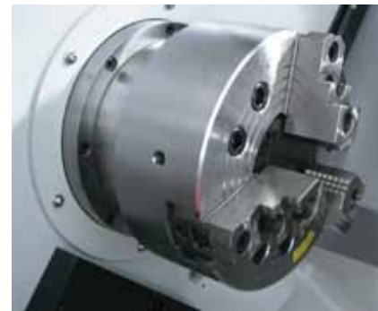
Hydraulic Chuck Fitting
