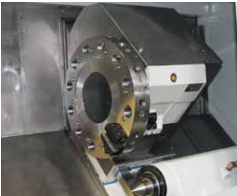
Hydraulic Type Turret w/ VDI Disc (Opt.)
