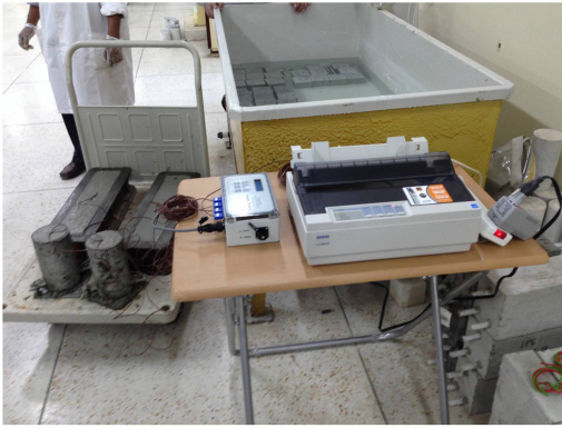
Plate 2. Connecting specimens to maturity meter.
