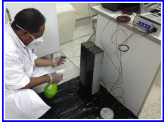
Plate 1. Application of spray coating curing.
