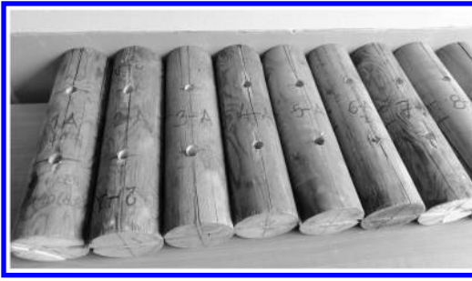
Figure 6. Round timber specimens before testing.
