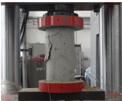
Figure 7. Failure modes of cylinders.
