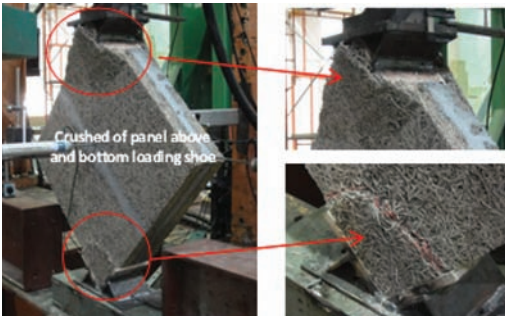
Figure 8. Failure mode of wallettes W2.
