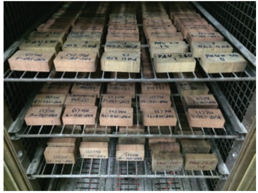
Figure 3. Sample placement in the oven.
