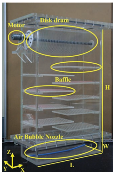
Figure 1. Experiment model in a water basin with baffle plates and rotating disks.
