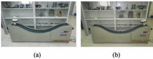
Figure 1. Slider machine that consistently shifts the antennas from positions (a) to (b) throughout the field observation.
