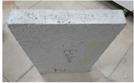
Figure 1. First sample with common concrete C25/30.
