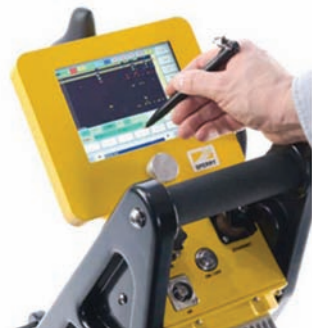
Figure 5. Portable ultrasonic equipment for rail inspection (Advances in Portable Ultrasonic Test Equipment).
