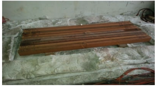
Figure 2. Arrangement of the samples inside the electrical furnace.
