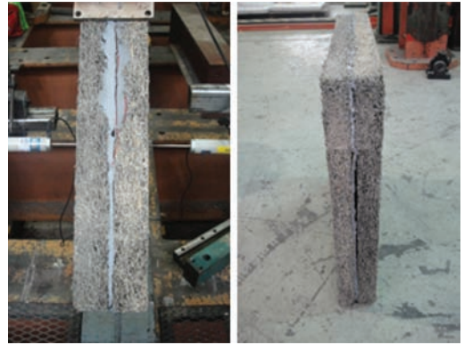
Figure 9. Vertical crack on the web of wallettes W2-S3 and W2-M5.
