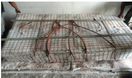
Figure 1. Specially designed electrical furnace made up from ceramic fiber.
