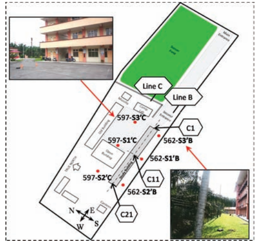
Figure 3. Positions of seismometer sensors on the ground surfaces in SK Sri Molek compound.
