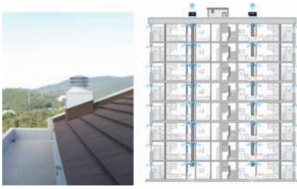
Figure 1. Power fan on the rooftop and the diagram of the fan-assisted hybrid ventilation system.
