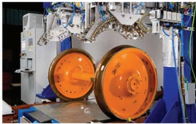
(a) Automated ultrasonic testing system (Automated Ultrasonic Railroad Wheel Set Inspection).
