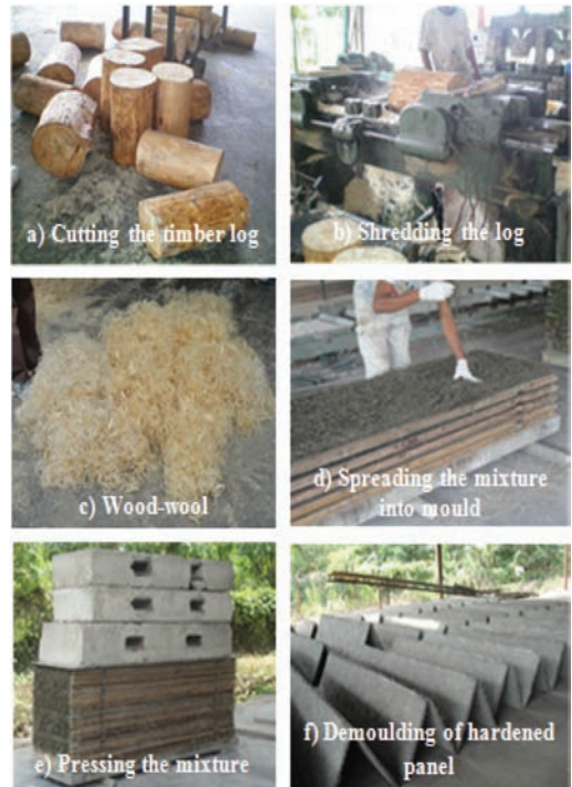
Figure 1. The production process of WWCP.
