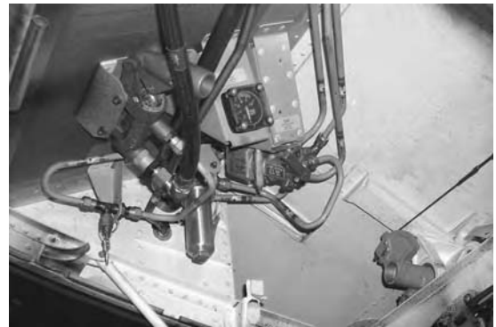
Figure 1.2 Boeing 767 hydraulic reservoir charging point, showing contents gauge, changeover valve and hydraulic hand pump.
