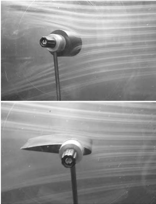
Figure 7.21 Smoke generator traces, showing differences in flow behind a cylinder and an aerofoil section. With subsequent reduction in form drag, as indicated in Figure 7.20.
