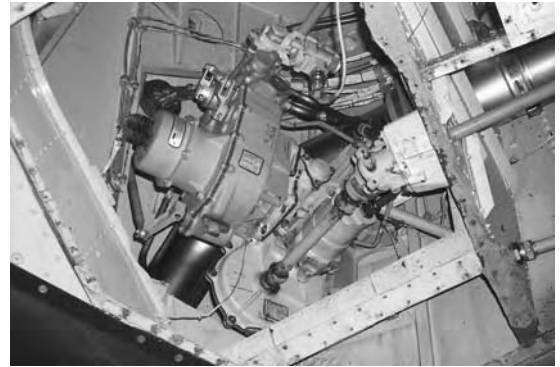
Figure 1.4 Boeing 767 flap drive motor and associated drive mechanism.
