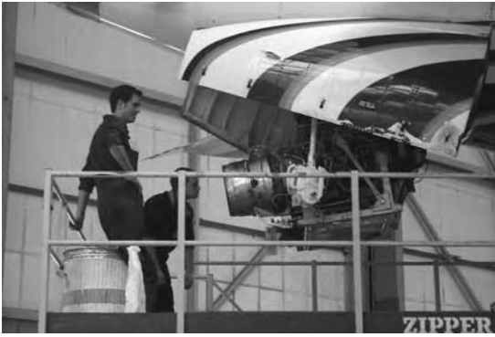
Figure 1.5 Technicians working at height considering the alignment of the APU prior to fit.
