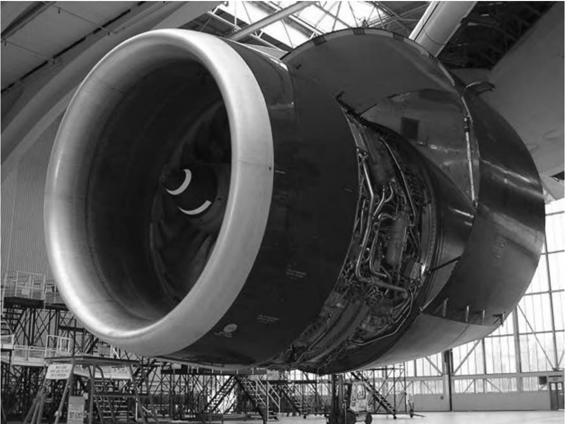
Roll-Royce RB211-524 Engine fitted to a Boeing 747 Aircraft
