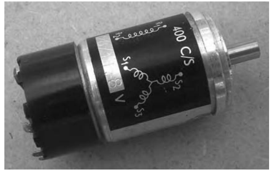
Figure 6.125 Typical arrangement of synchros in an aircraft instrument.
