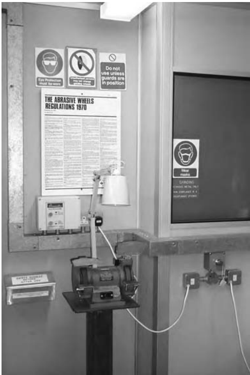
Figure 1.19 Grinding wheel assembly, with associated lighting and warning signs.
