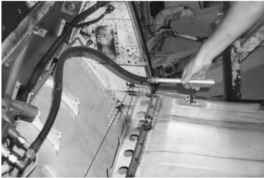
Figure 1.3 Hydraulic reservoir replenishment hose, removed from stowage point.
