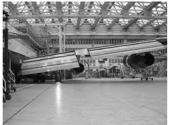
Figure 7.63 Trailing edge multi-slotted Fowler flap system on Boeing 747-400.
