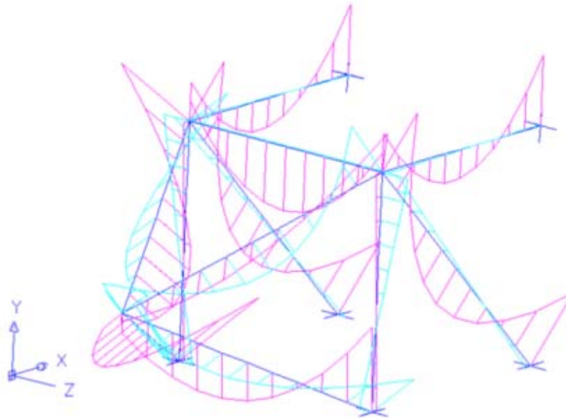
Figure 11.6: Diagram of bending moment-Z and bending moment-Y are displayed together
