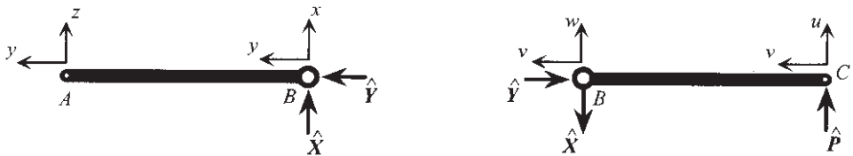
Figure 4.19 System of two, originally motionless straight rods, AB, BC ( C : hinged; A, B, C : collinear) struck by a blow \hat{P} at its end C , at a right angle to ABC , specially relaxed at B in order to calculate the internal reactions there.
