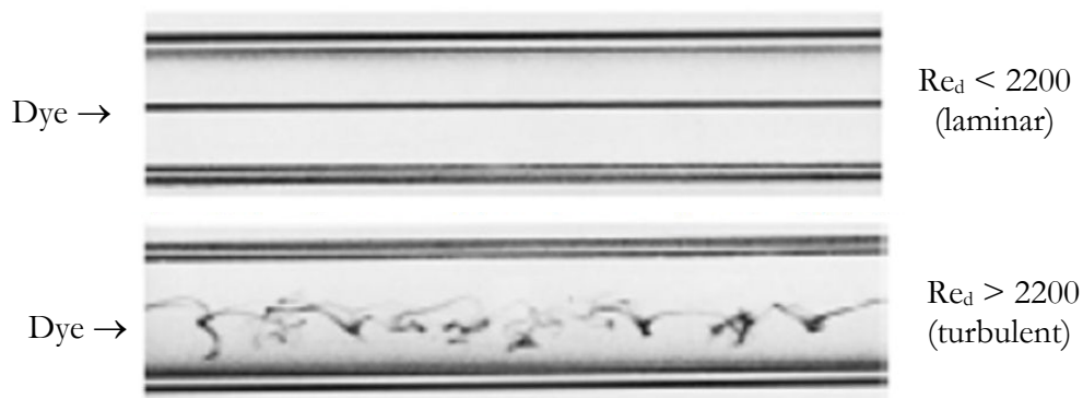
Figure 19. Images of a tracer dye in laminar and turbulent pipe flow. Flow from left to right. (From M. VanDyke, “An Album of Fluid Motion,” Parabolic Press, 1982.)
