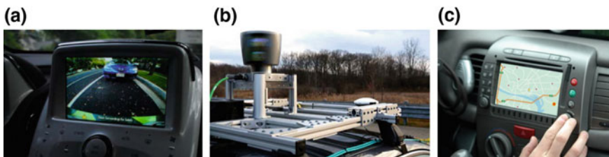
Fig. 2 Vehicle implementation of currently available CAV technologies: a CS, b LiDAR [6], and c GPS [7]
