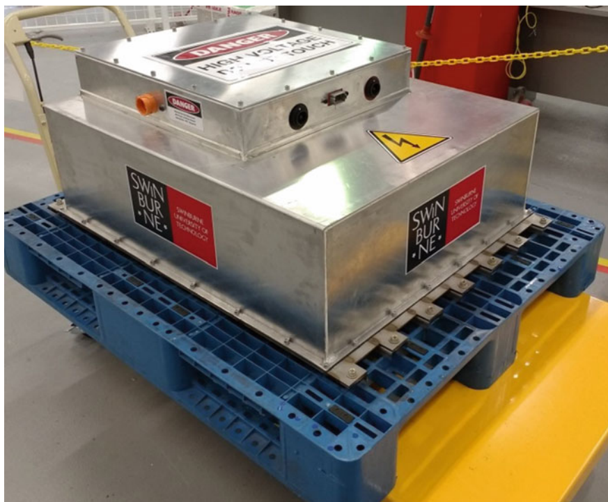
Fig. 9 Complete battery pack ready for fitment to bus
