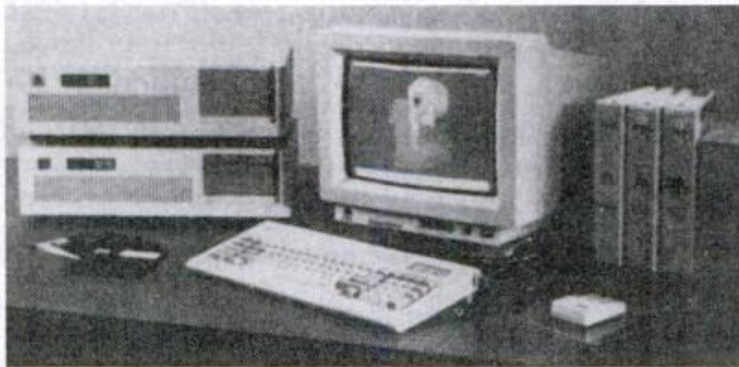
Fig. 2.37 Desktop MCAE System Based on an Enhanced IBM PC/AT. ( Courtesy of Aries Technology, Inc. )
