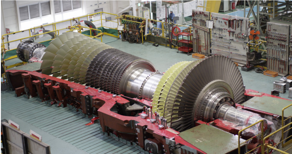
Figure 3.1 A Mitsubishi-Hitachi M701J on the factory floor. Source: Reproduced by permission of Mitsubishi Hitachi Power Systems, Americas, Inc.
