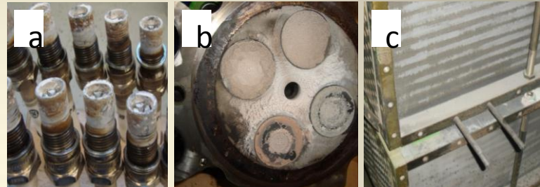
Deposits formed in landfill gas engines: a.spark plugs, b.engine head, c. intercooler radiator (Sevimoglu and Tansel, 2012).
