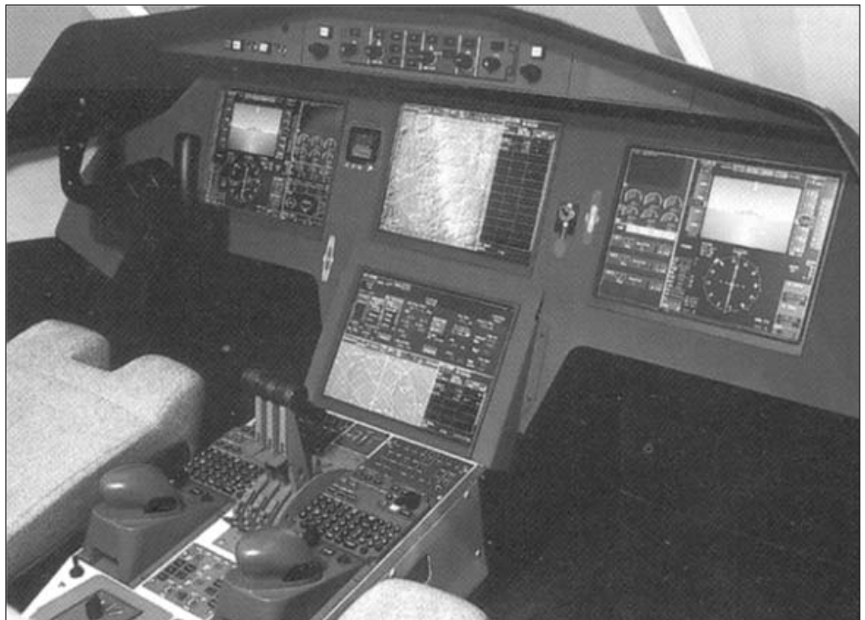
Fig. 7.45 Conceptual flight deck with four 13 x 11 inch displays
