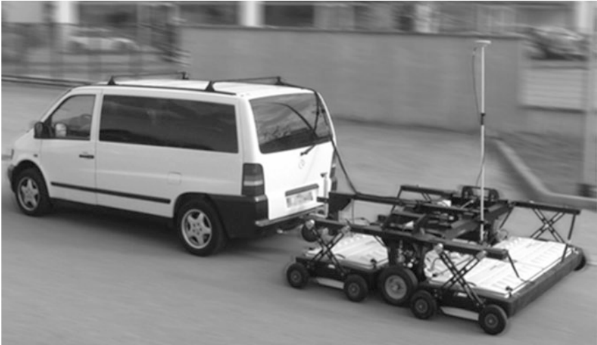
Fig. 11 A dense array GPR for the detection of underground assets (IDS Stream EM)
