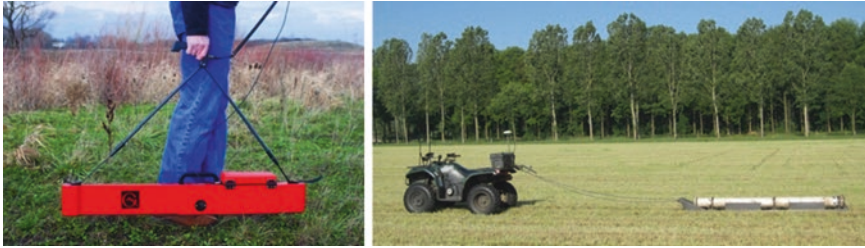
Fig. 5 Two mobile configuration of an EMI sensors. Left the handheld EM38–MK2. Right the Dualem-21S inside a towed sled
