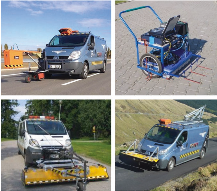
Fig. 2 GPR systems for road diagnostics—a two-channel pulse radar system with a combination of ground coupled and air coupled antennas ( upper left ), a cart for measuring the position of dowels and tie bars with two ground coupled antennas ( upper right ), stepped frequency systems for 3D measurements—ground-coupled ( lower left ) and air-coupled ( lower right ). Source Roadscanners, cart—CDV
