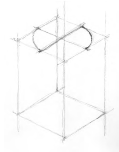
Figure 14.11: Drawing an isometric cylinder. Step 2.
