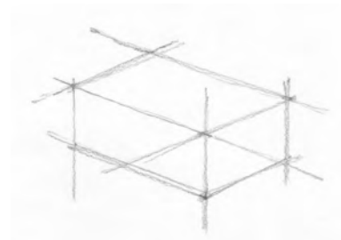
Figure 14.7: Drawing an isometric prism with hidden edges. Step 1.
