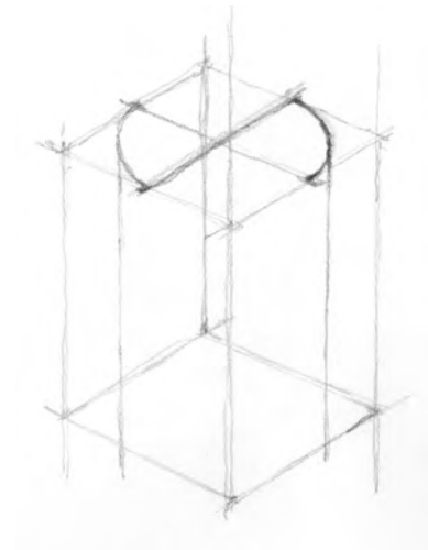
Figure 14.12: Drawing an isometric cylinder. Step 3.
