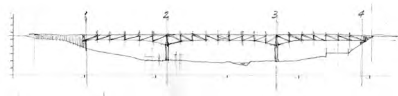
Figure 5.11: Bridge over a valley: truss concept
