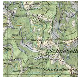
Figure 10.14: National Map of Switzerland ( Landeskarte der Schweiz ) 1:50 000 (to scale). Each square represents 1 km. Contour interval is 20 m.
