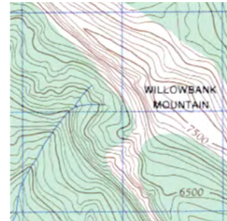
Figure 10.13: Canadian National Topographic System 1:50 000 (to scale). Each square represents 1 km. Contour interval is 100 feet (about 30 m).
