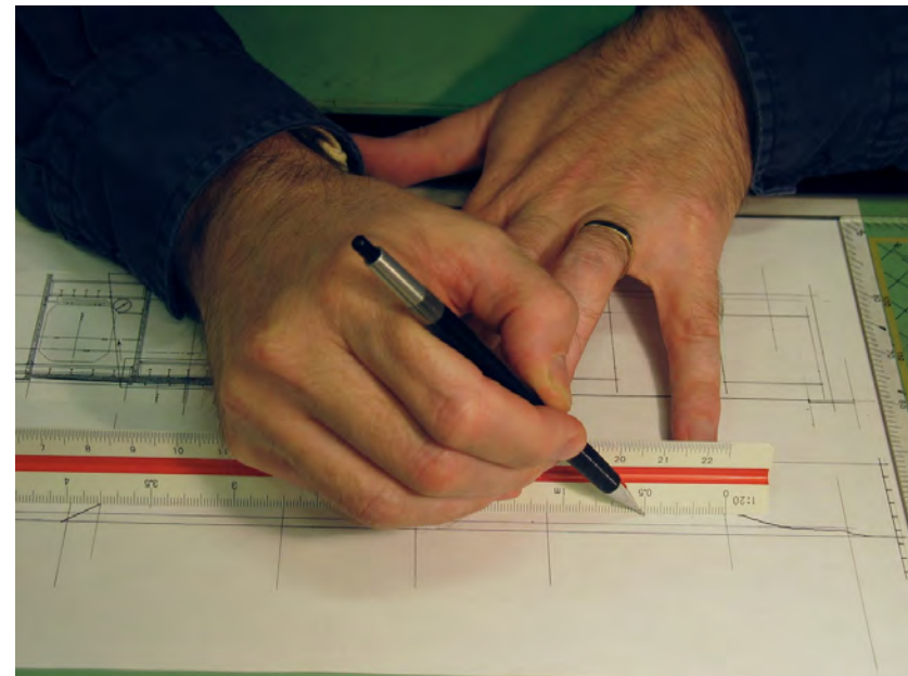
Figure 9.5: Creating a drawing using a metric scale . Note the ratio 1:20 imprinted on the scale. The distance measured is a power of 10 times 0.5 m.
