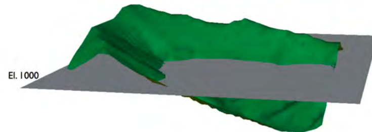
Figure 10.4: Landform of Figure 10.1 sliced by a plane at Elevation 1000
