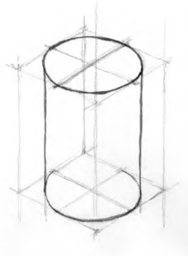
Figure 14.14: Drawing an isometric cylinder. Step 5.
