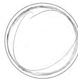
Figure 11.4: The corrected freehand circle of Figure 11.3 with a “perfect” circle drawn using CAD
