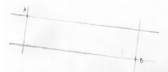
Figure 13.14: Drawing a long straight line between two given points: Step 3
