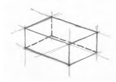
Figure 14.9: Isometric prism showing both visible and hidden edges.
