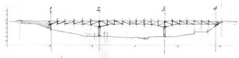
Figure 5.14: A more precise sketch of the truss concept (reproduced from Figure 5.11)
