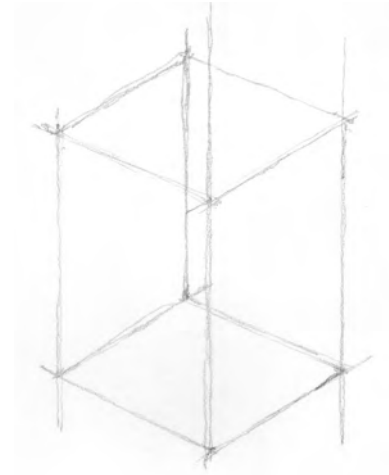
Figure 14.10: Drawing an isometric cylinder. Step 1.
