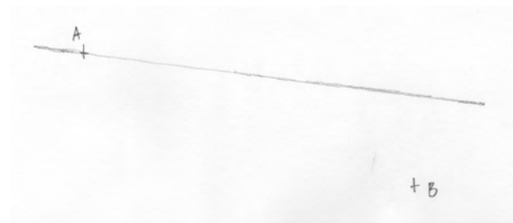
Figure 13.12: Drawing a long straight line between two given points: Step 1
