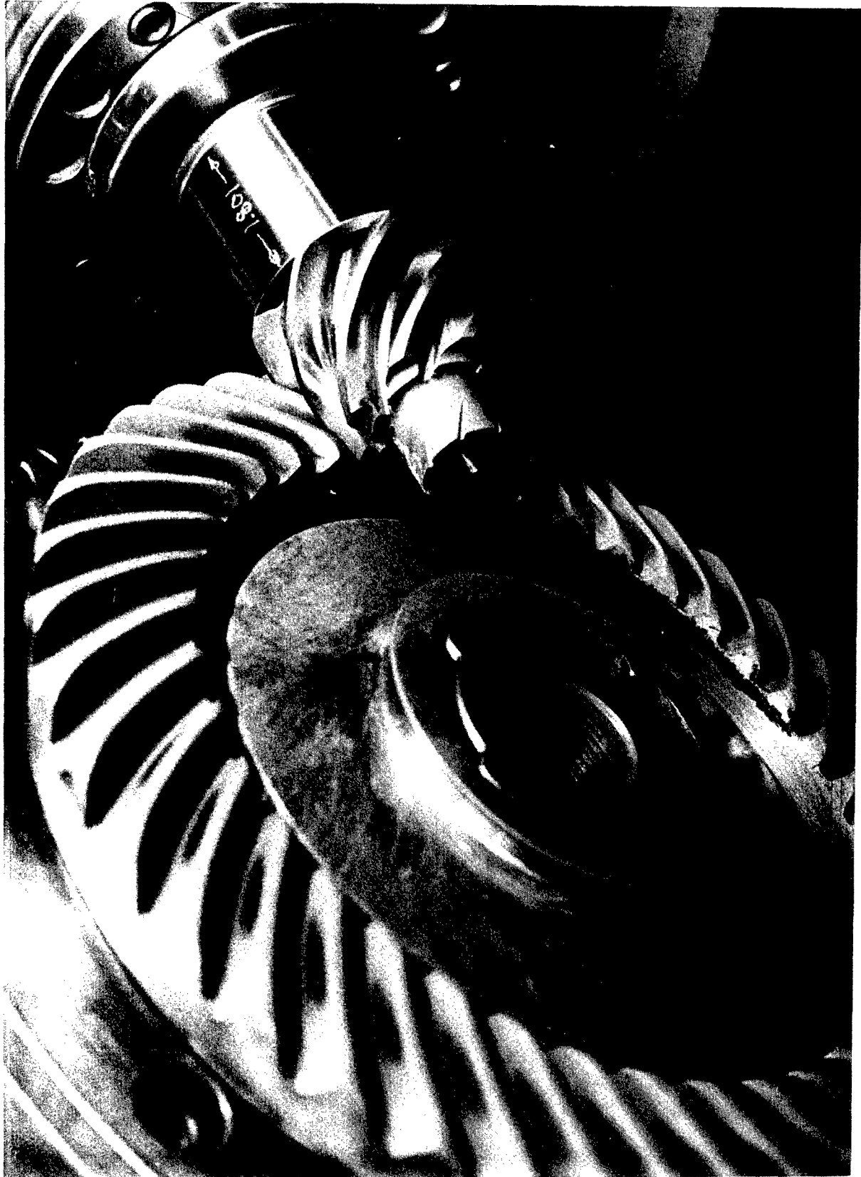
FIGURE C-8. Tooth Contact Pattern of Net Forged Gear (From the Third Series of Trials) and Machined Matching Pinion
