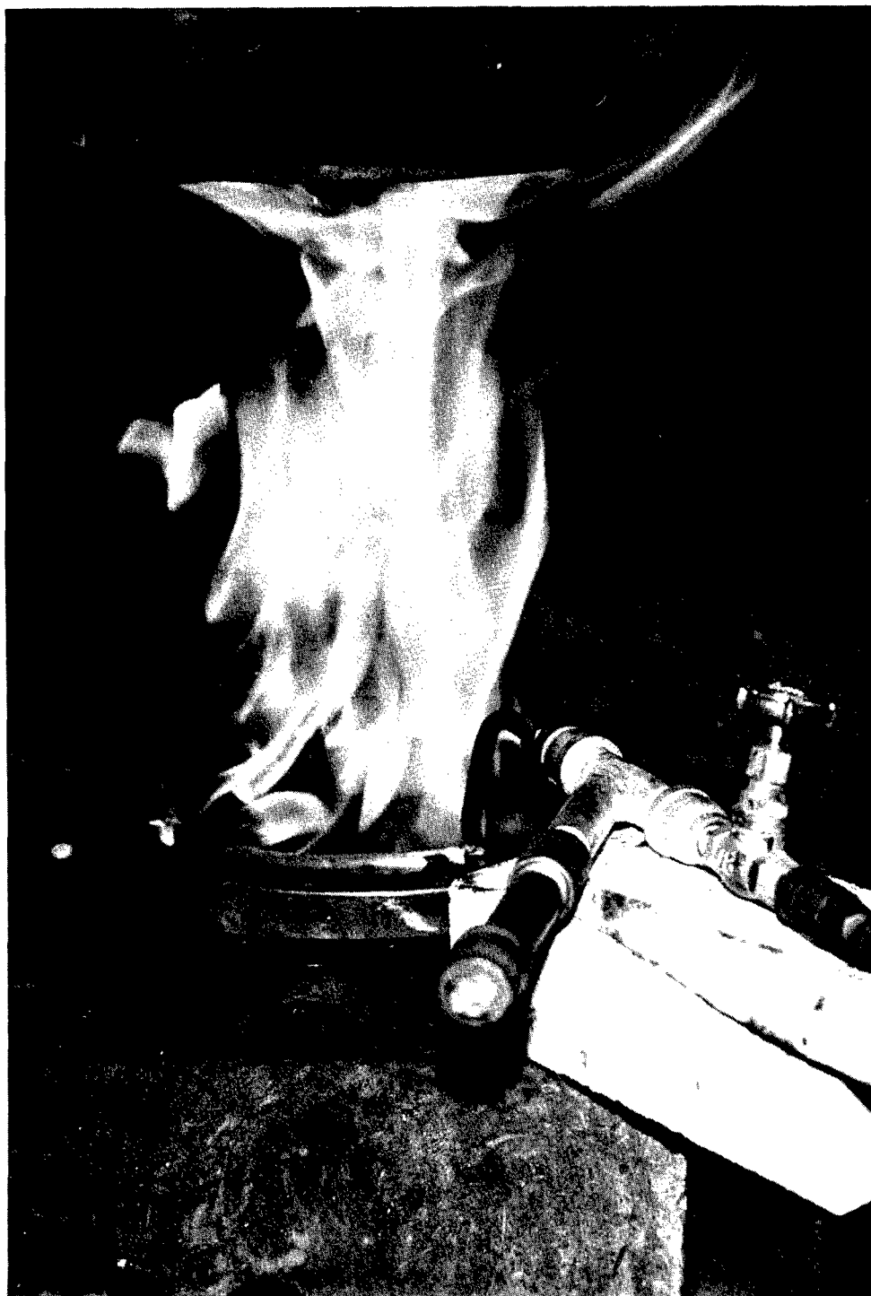
FIGURE B-7. Heating of the Dies With a Circular Gas Flame
