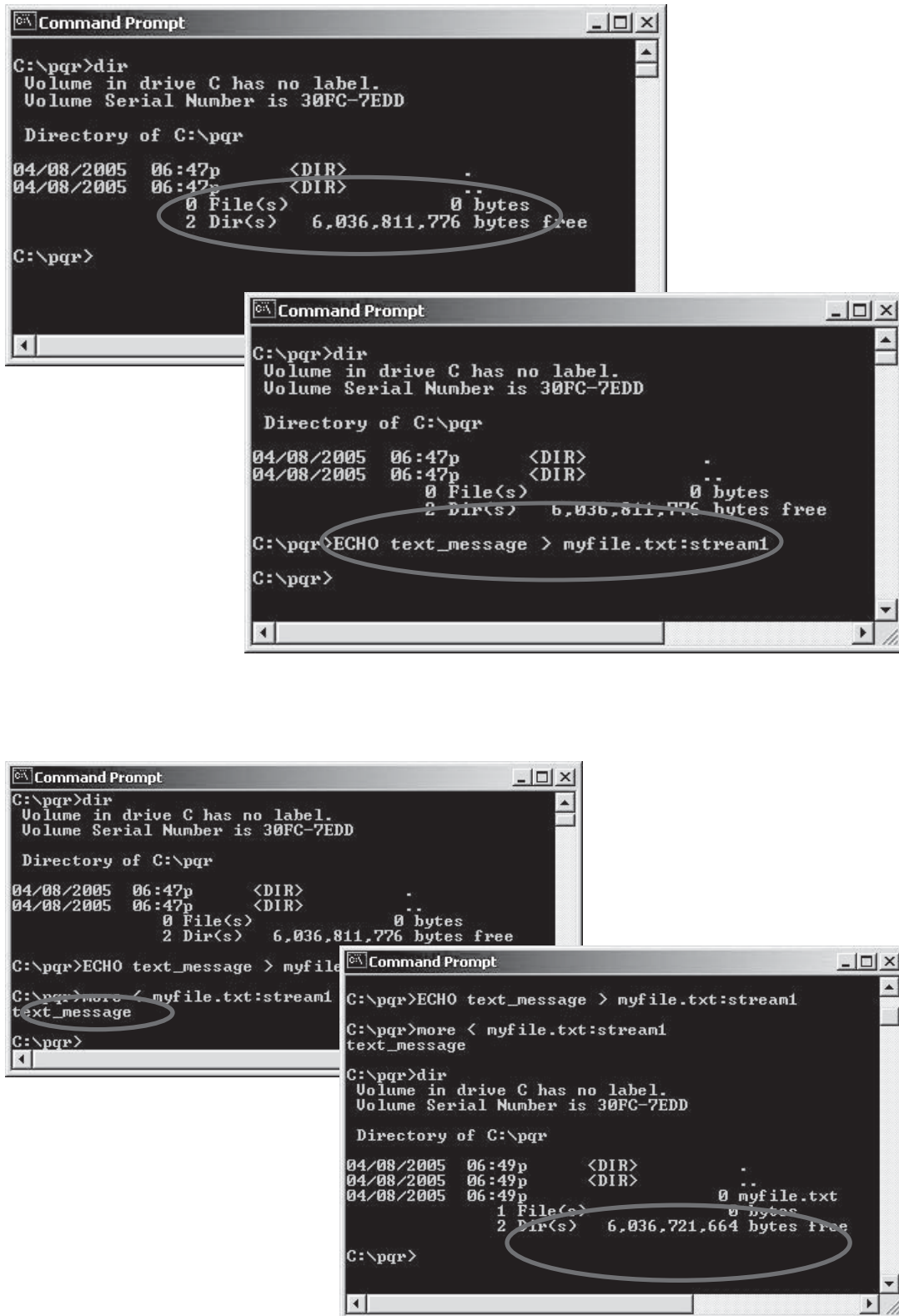
Figure 1-10 A user can create and examine data streams using the command line
