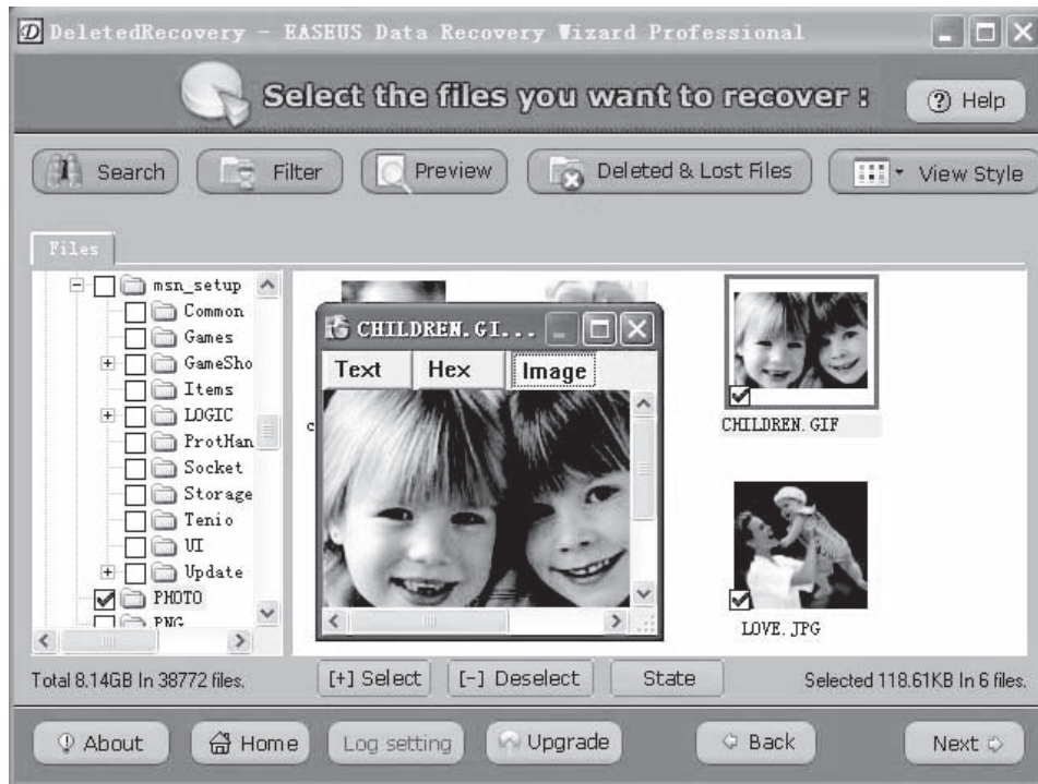
Figure 11-1 Data Recovery Wizard allows investigators to recover files a suspect has deleted.
