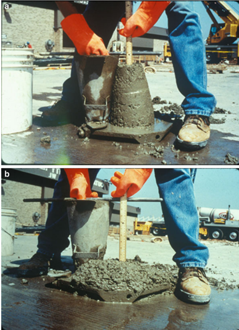
Figure 1.5 Slump test (courtesy of Portland Cement Association)
