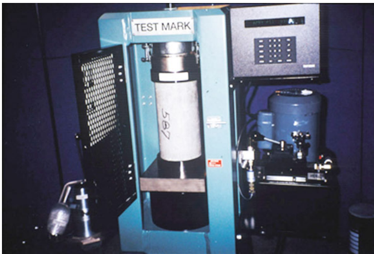
Figure 1.7 Cylinder test (Courtesy of Portland Cement Association)
