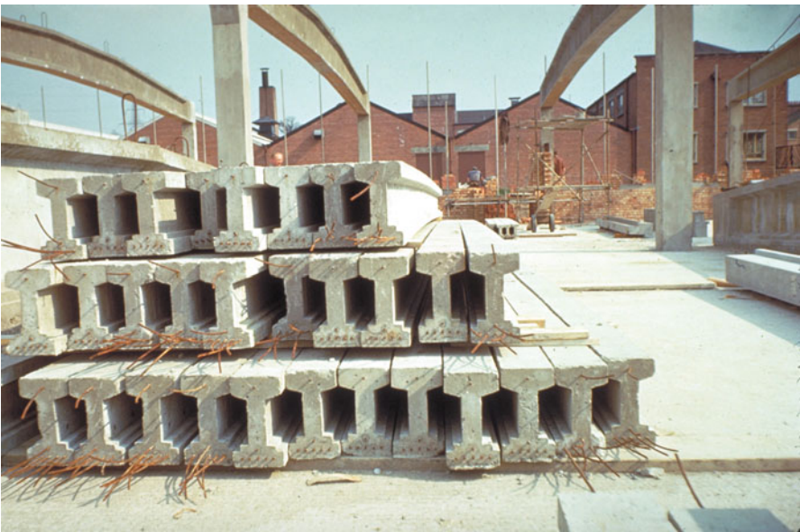
Figure B9.1 Prestressed I-Section concrete beams Courtesy of the William G. Godden Collection, NISEE-PEER, University of California, Berkeley
