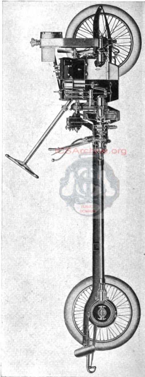
Fig. 29. Vertical Section of Briscoe Chassis Courtesy of Briscoe Motor Company, Jackson, Michigan
