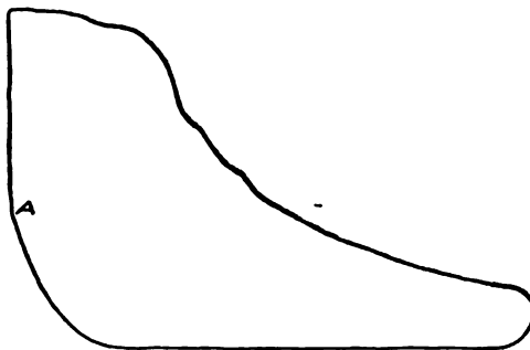
Fig. 15. Actual Indicator Card, Showing Compression
