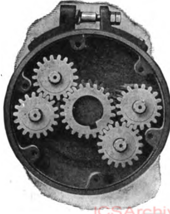
Fig. 52. Forward View of Buffalo Reverse Gear Courtesy of Buffalo Gasoline Motor Company, Buffalo, New York
