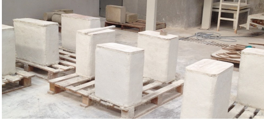
Figure 2.16: Columns with rectangular cross-section after confinement.
