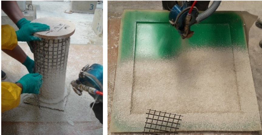
Figure 2.3: Application of GFRC with sprayed-up method.
