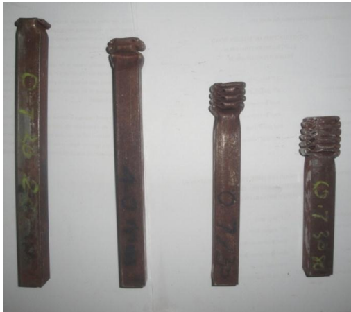
Figure 3: Results from the impact load test
