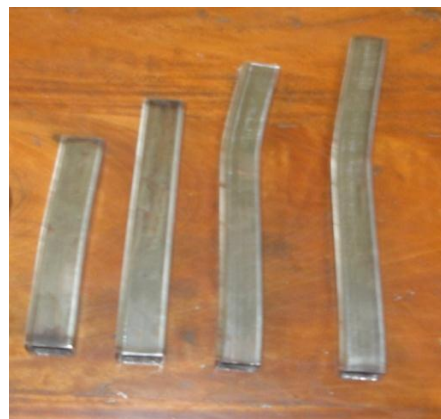
Figure 2: Results from the static compression test
