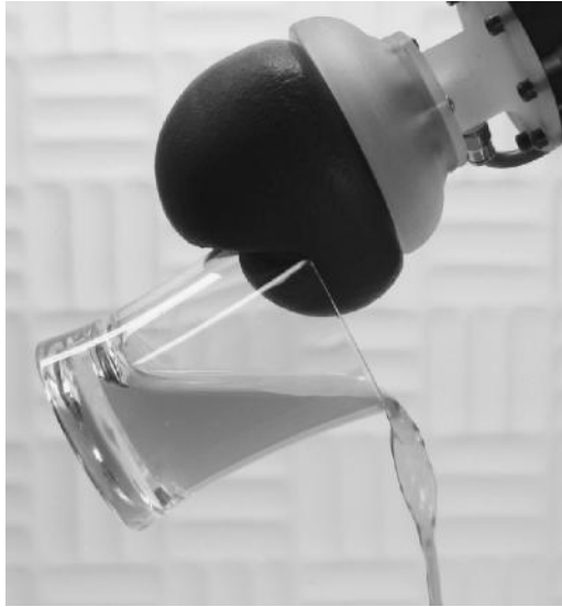
FIGURE 9.4 Highly specialized end effector.
