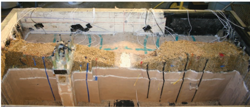
Fig. 12.15. Photograph of the centrifuge model during dissection; note that the pile cap displaced 0.75 m (prototype) toward the channel while the opposing embankment crest displaced 1.7 m (prototype) toward the channel
