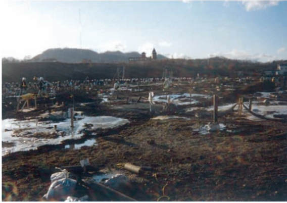
Fig. 15.4. Liquefaction induced by subsoil blasting in Tokachi Harbor
