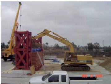
(c) Bridge abutment soil model construction on shake table
