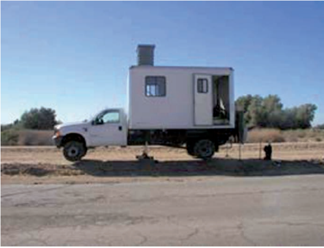
Fig. 5.14. Cone penetration testing truck
