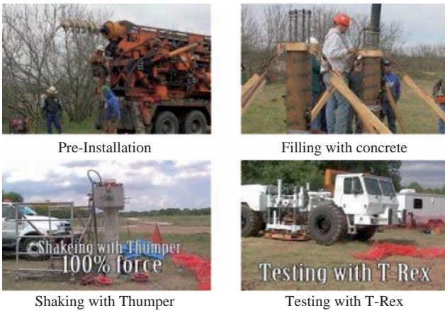
Fig. 5.22. Field test model construction and dynamic excitation ( http://nees.utexas.edu )
