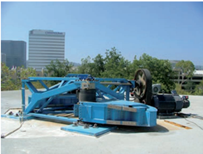
Fig. 5.11. MK-15 eccentric mass shaker during UCSD Elliot Field testing
