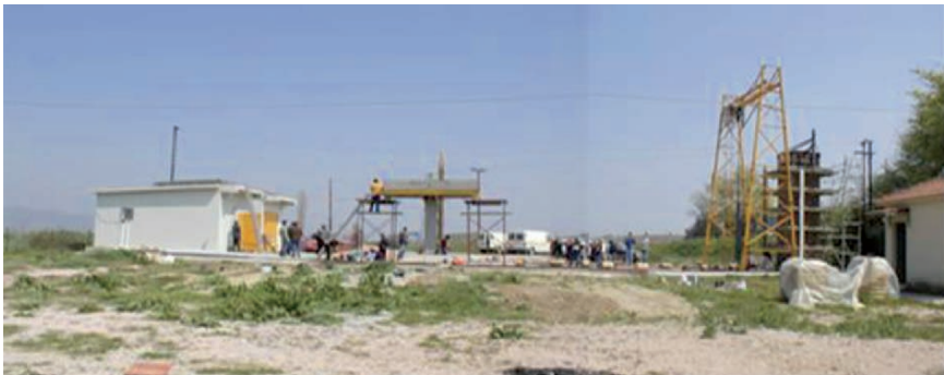
Fig. 5.5. Experimental field facilities to study SSI effects and the behaviour of RC. structures (Instrumented five-storey RC building with masonry in fills and a pier bridge on surface foundation, models' scale 1:3)
