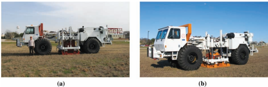
Fig. 7.1. Large mobile vibrators used as controllable, high-energy seismic sources: (a) the low-frequency vibrator called Liquidator and (b) the tri-axial vibrator called T-Rex
