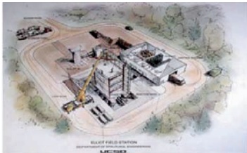
(a) Facility layout including shake table and adjacent large soil pit
