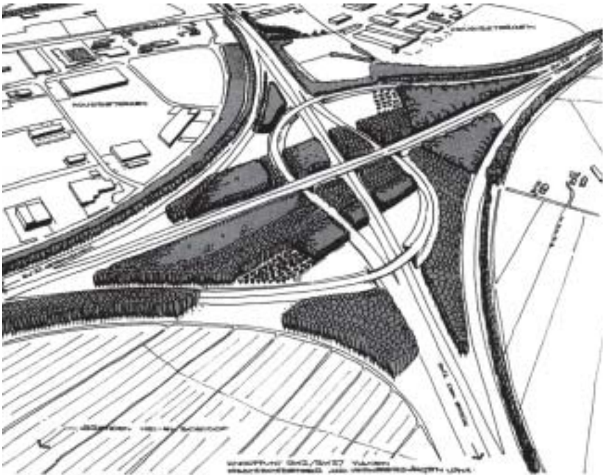
Figure 3. The layout of the Vianen junction is an example of a layout that, while being related to the surroundings, has a more autonomous monumental shape with large 'tree-meadows' with oaks, and poplars in particular, forming a 'green' portal to the Randstad (design by Nas, Elffers and Meijer).
